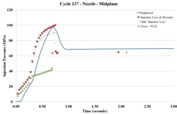
Figure 4 – Injection pressure profile comparison for Cycle 237, using the midplane solver.
