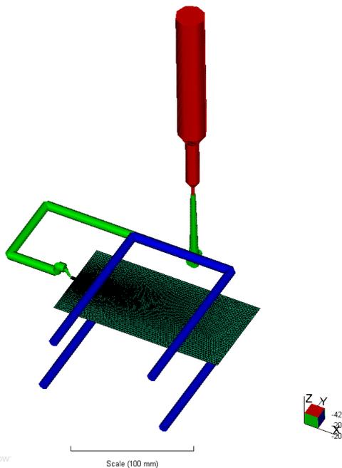
Figure 2– A representation of the midplane model used for the simulations, which modeled the entire mold design including the machine nozzle (red) and cooling circuits (blue).
