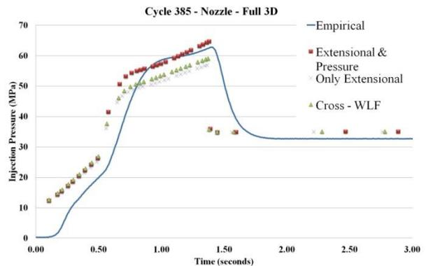
Figure 9 – Injection pressure profile comparison for Cycle 385, using the full 3D solver.
