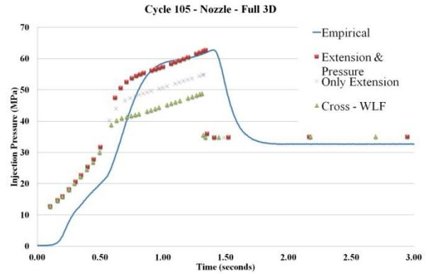
Figure 7 – Injection pressure profile comparison for Cycle 105, using the full 3D solver.
