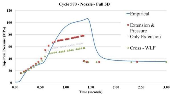
Figure 10 – Injection pressure profile comparison for Cycle 570, using the full 3D solver.
