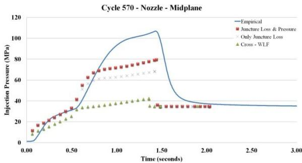
Figure 6– Injection pressure profile comparison for Cycle 570, using the midplane solver.
