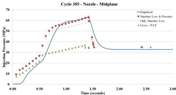
Figure 5– Injection pressure profile comparison for Cycle 385, using the midplane solver.
