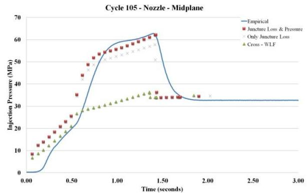
Figure 3– Injection pressure profile comparison for Cycle 105, using the midplane solver.
