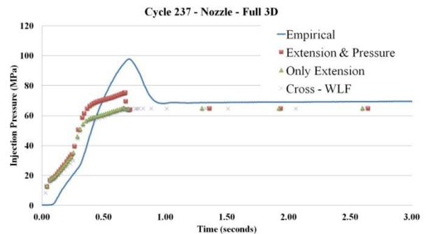
Figure 8 – Injection pressure profile comparison for Cycle 237, using the full 3D solver.
