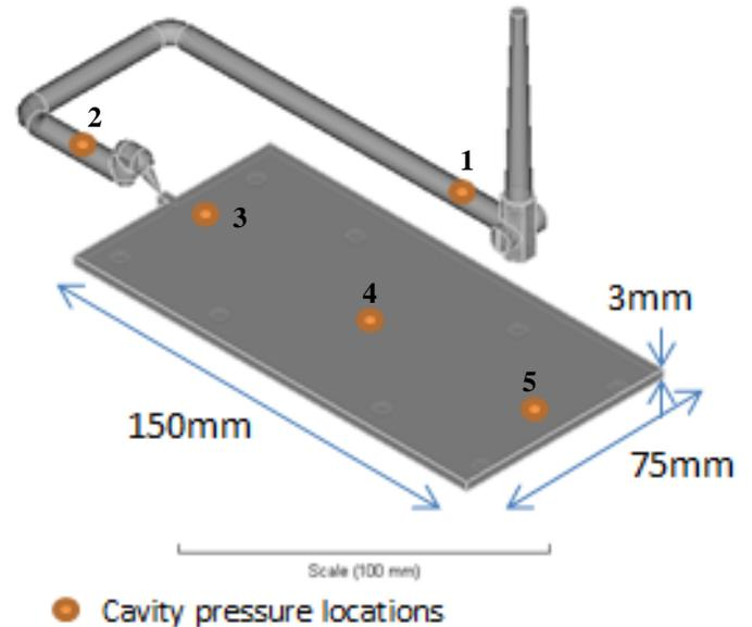
Figure 1 – Schematic showing the location of the pressure sensors within the plaque mold.
