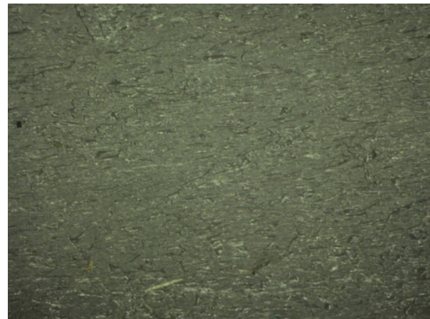
Figure 6: Rough surface finish caused by fibers on the surface of the part
