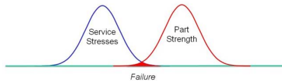
Figure 2: stress and strength distributions overlapping leading to a failure probability
