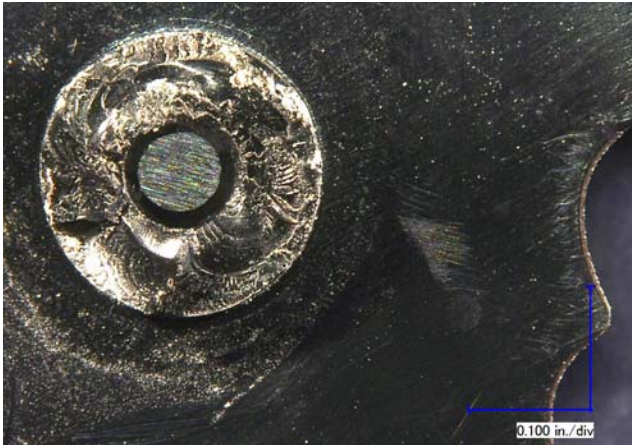
Fig. 1 - The fracture surface from one of the failed panel bosses is shown exhibiting features characteristic of brittle fracture. Multiple individual crack origins are present around the inner diameter of the boss.
