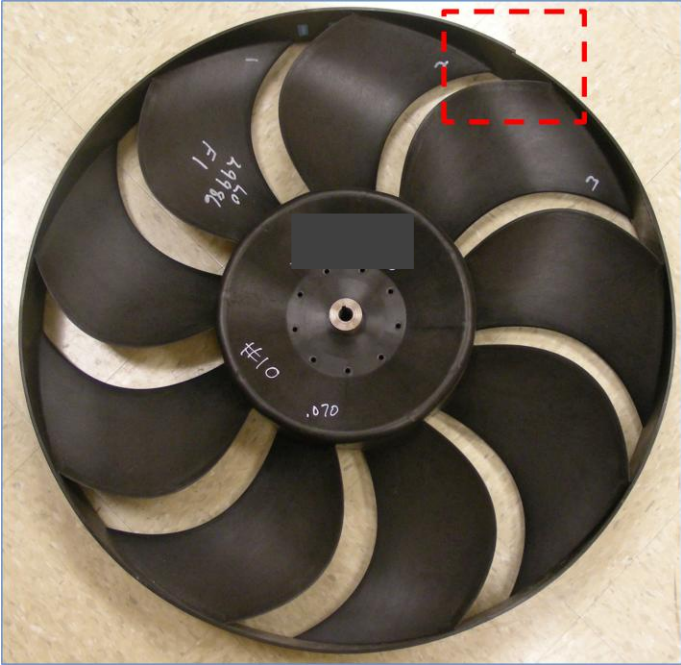
Figure 7 – Industrial fan analyzed with DMA for lifetime prediction.
