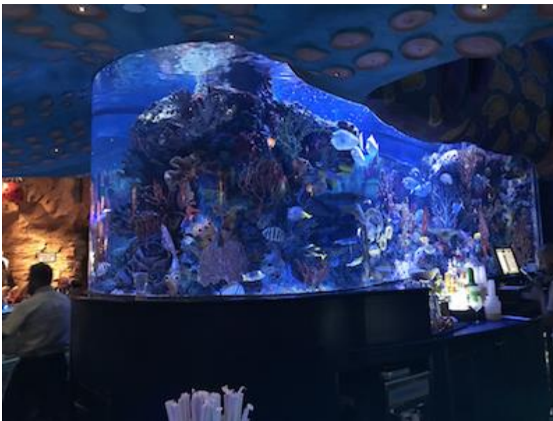
The aquarium at the T-Rex restaurant at Walt Disney World in Orlando, FL, failed in 2014, when a vertical bonded seam opened instantaneously. Image courtesy Paul J. Gramann.
