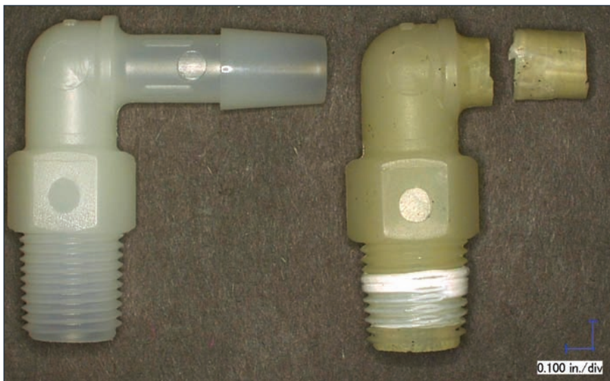
Figure 2: Reference and failed connectors, shown as received. The failed parts exhibited significant discoloration.
