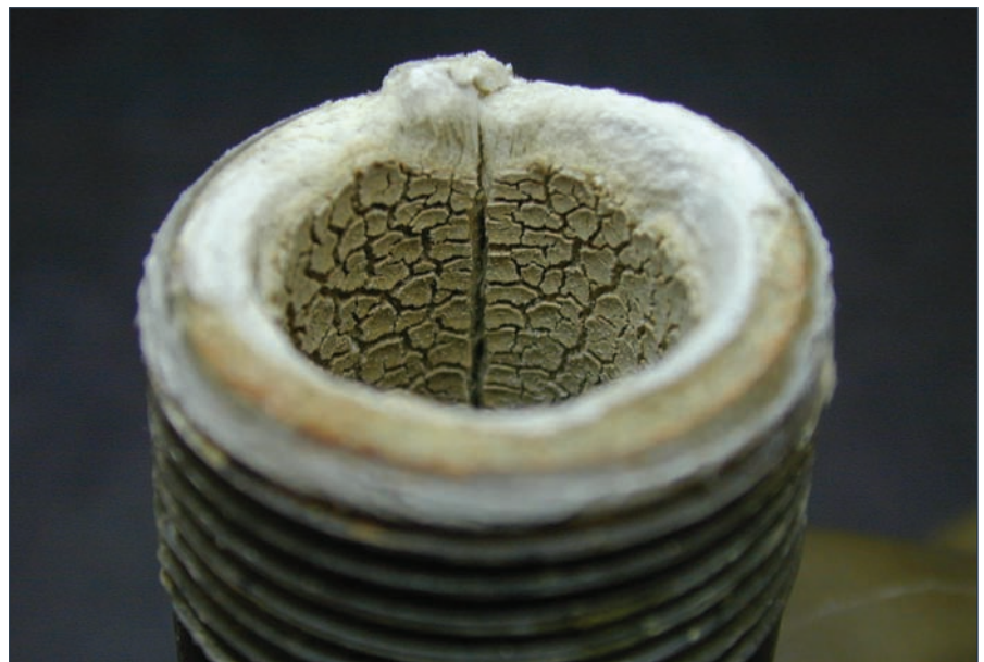
Figure 1: This nylon water-heater valve degraded through contact with chlorinated water at elevated temperatures.
