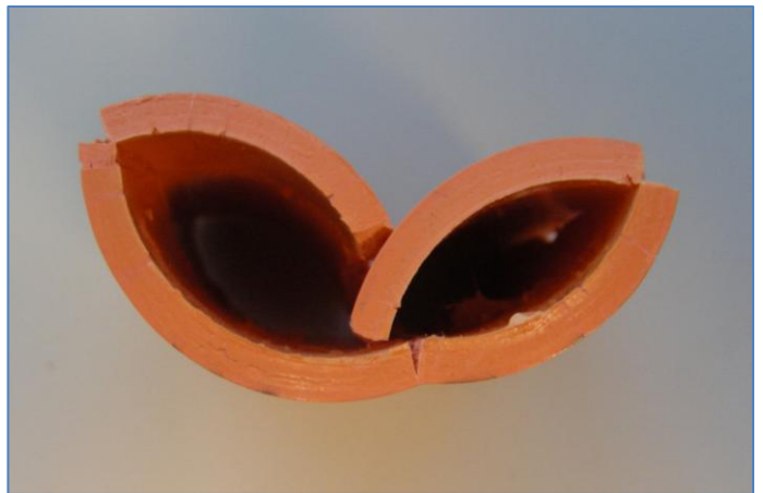
Figure 9 – Result of flattening test [8] of a CPVC section that was exposed to a mixture of water and bio-glycerin.
