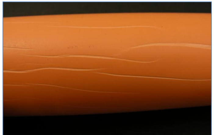
Figure 5 – Axial striations on the outside a failed CPVC pipe exposed to a mixture of water and bio-glycerin.
