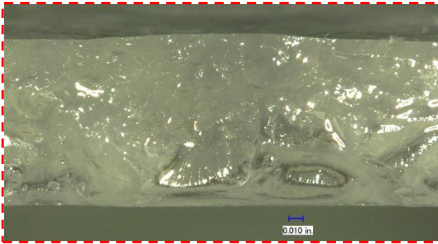
Figure 5 – Fracture surface of a polycarbonate sample after exposure to biodiesel and 1.5% strain.
