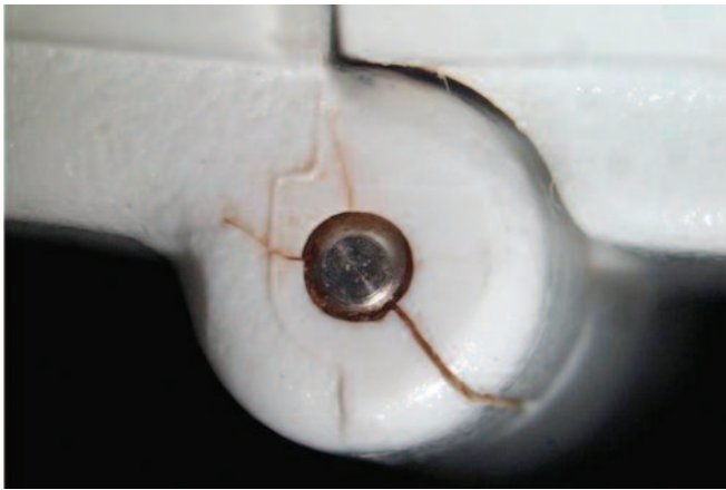
Cracking was present within the housing of a personal medical monitor (left). The features were characteristic of brittle fracture, with no discernible ductility. The scanning electron microscope image (right) shows a typical fracture surface on the medical monitor, with characteristics of brittle fracture through low cycle fatigue.
