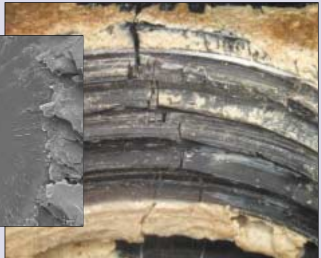
Fig. 5—Images illustrate the cracking in the sprinkler housings.
