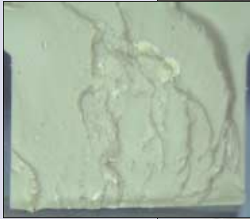
Fig. 3—Photomicrographs show the crack location within the hinge and the fracture surface.
