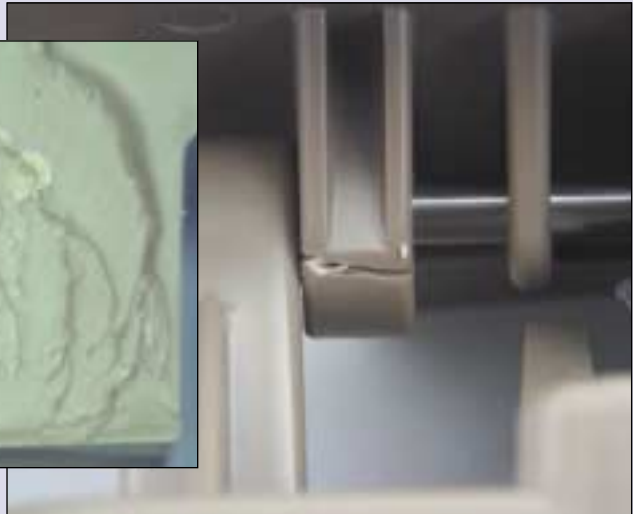
Fig. 3—Photomicrographs show the crack location within the hinge and the fracture surface.
