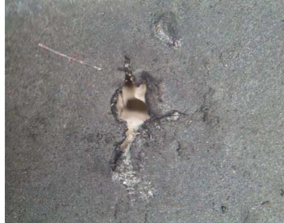
Figure 7 – White included contaminant material was present within the hose cover layer.
