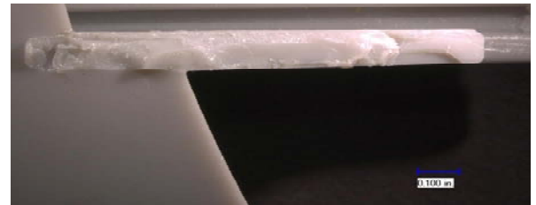
View of the fracture surface of a typical failed actuating lever. Multiple individual cracks are evident. The fracture surface shows no signs of ductility.
