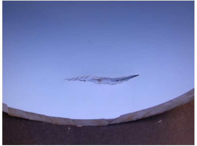
Figure 2 – Circumferential crack in PVC pipe prior to installation.
