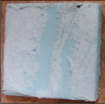
Figure 6 – PVC sample of failed Pipe #1 after immersion in dichloromethane.
