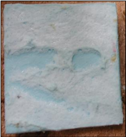
Figure 8 – PVC sample of failed Pipe #2 after immersion in dichloromethane.
