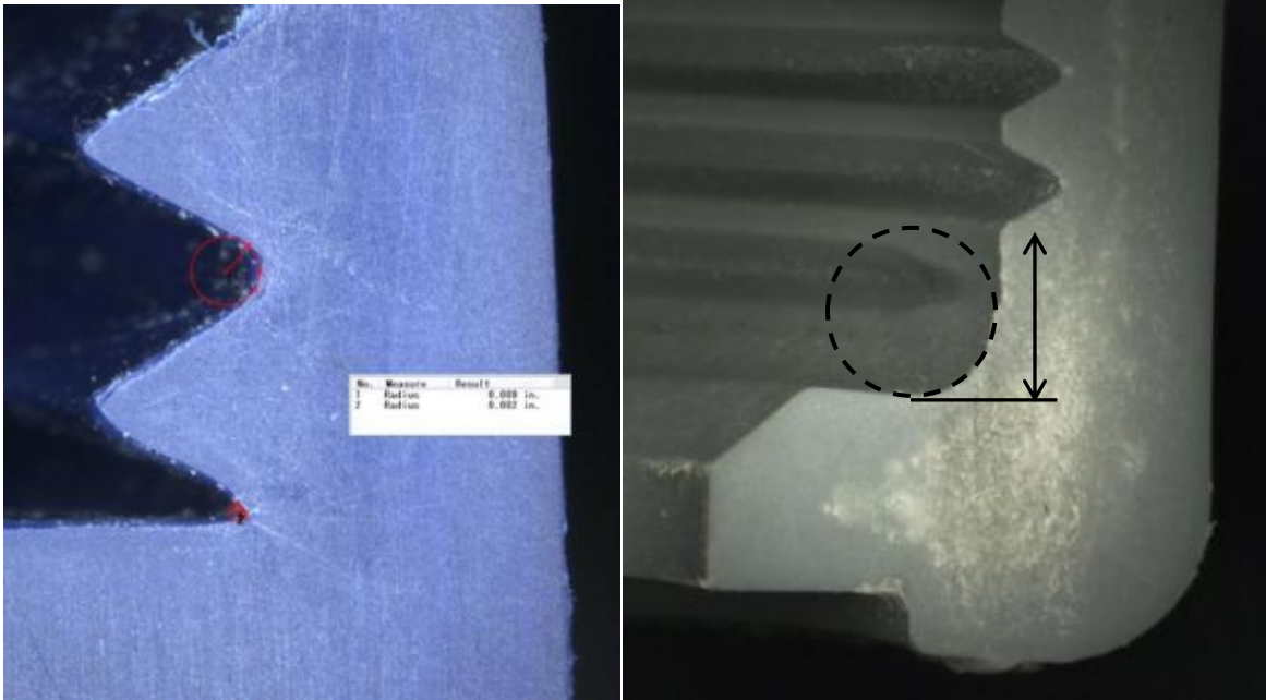
Figure 3 – Example of threads terminating at flange (left: termination directly into flange; right: termination away from flange and large radius)
