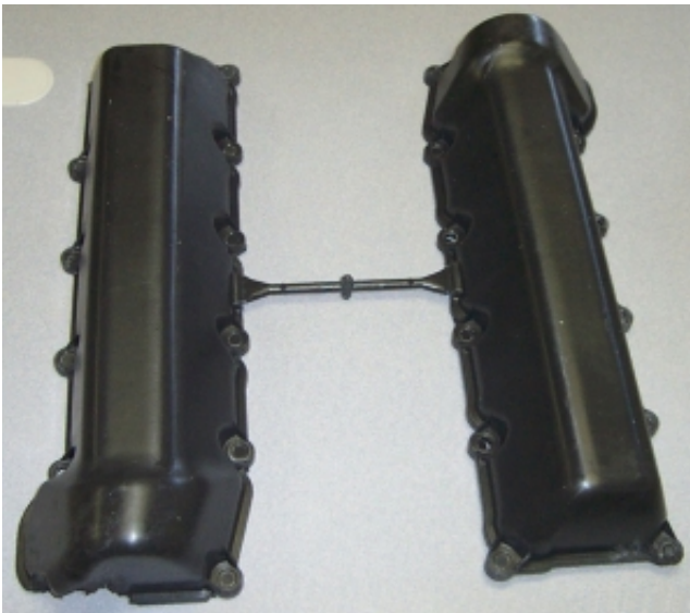
Figure 7. Left and right sides of 4.7L valve cover showing runner.
