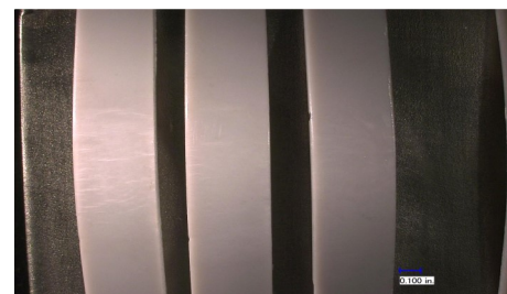
ESC testing showed cracking in the lever material when in contact with the sanitizing agent while under stress.
