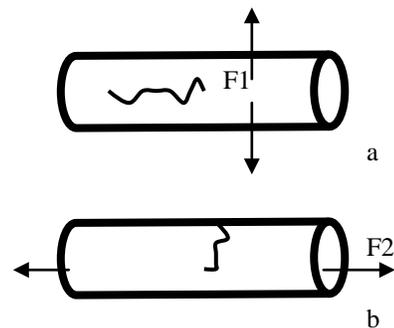
Figure 3 – Longitudinal cracking (a) and circumferential cracking (b) are illustrated within a pipe.
