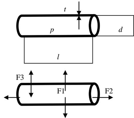
Figure 2 – The three principal stresses on the pipe wall are illustrated.
