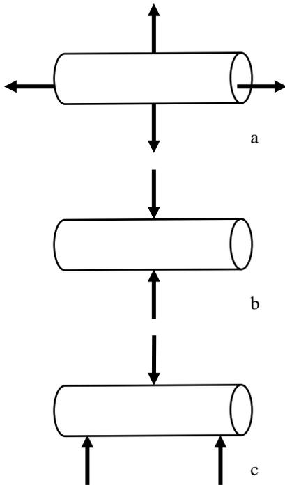
Figure 1 - Pipe loading demonstrating tensile stress (a), compressive stress (b), and bending stress (c).
