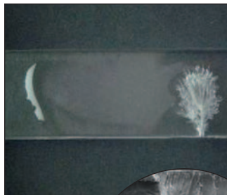
Fig. 7— Environmental stress cracking is shown with a polycarbonate resin.
