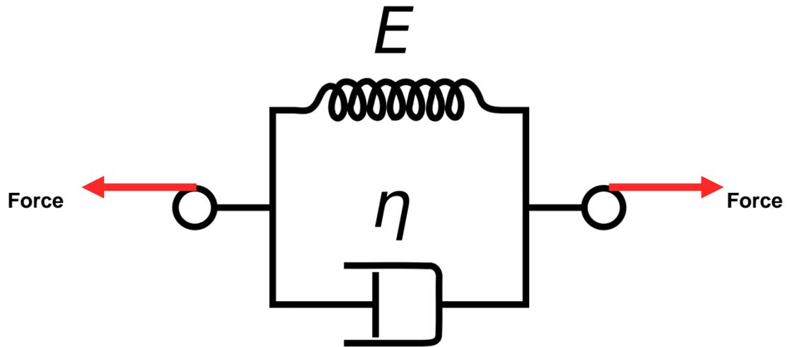
Figure 3. Damper and spring put in parallel configuration (Kelvin-Voigt model) to model the viscoelastic behavior of plastics [1].
