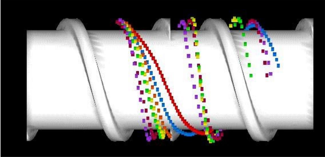
Figure 6, Particle tracking in the Inside-Out mixer
