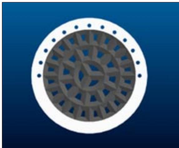
Figure 5 – Radial slotted MBP with guide holes for stacking plates in series.
