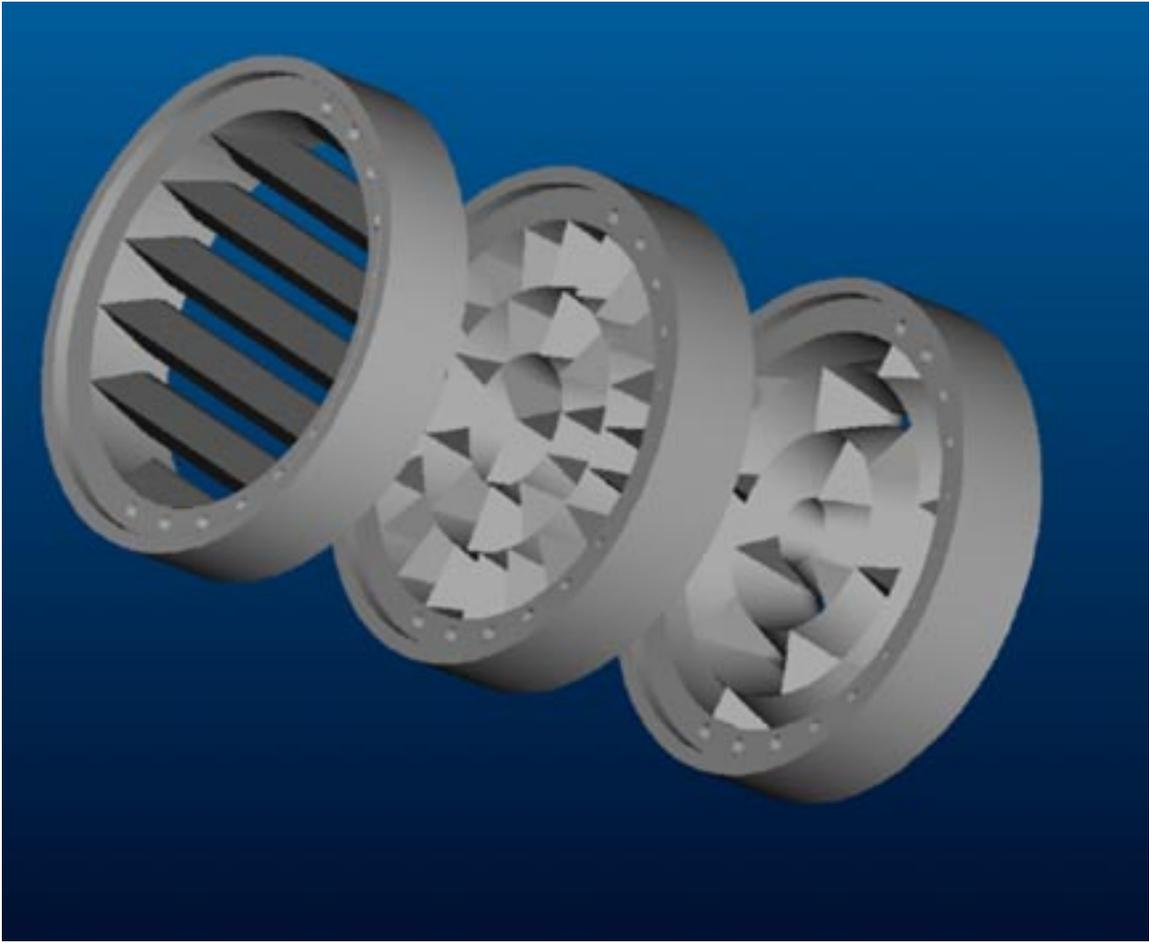
Figure 6 – Parallel, radial, and circular MBPs placed in series to create the dispersive/distributive static mixer (DDSM).
