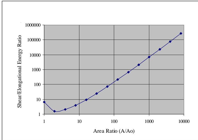
Figure 1 - Energy ratio (shear/elongational) required to produce dispersed phase of a specific size.
