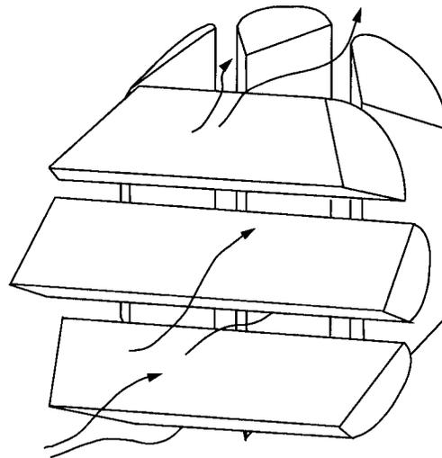
Figure 2 – General shape of converging wedges that create elongational flow.
