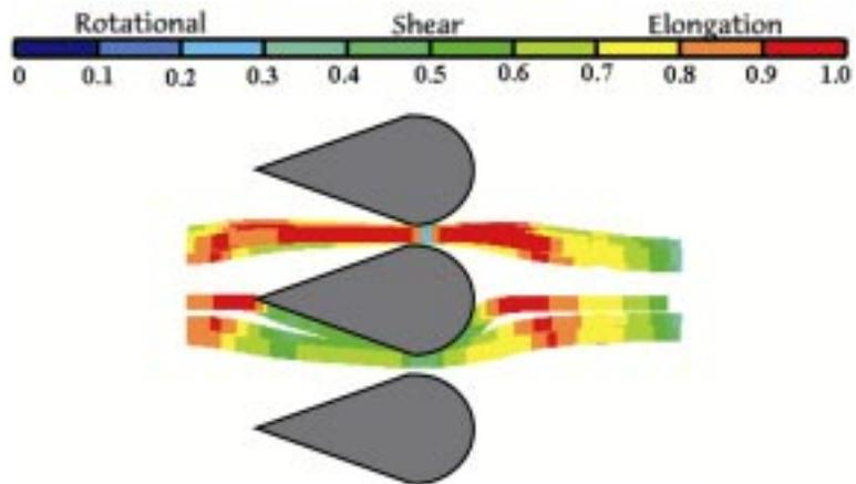
Figure 8 - Calculated flow number for particles tracked through they Mixing Breaker Plate (MBP).
