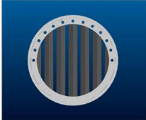
Figure 3 – Parallel slotted MBP with guide holes for stacking plates in series.
