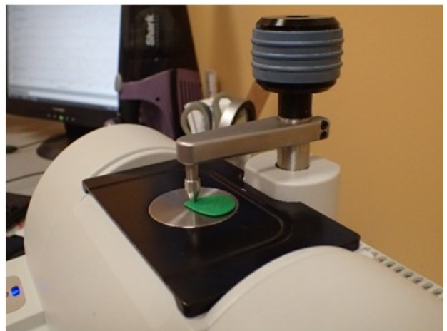
Figure 3 —FTIR Testing of guitar picks.
