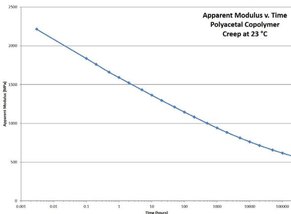
Figure 7. The plot of apparent modulus over time is shown for the polyacetal copolymer.
