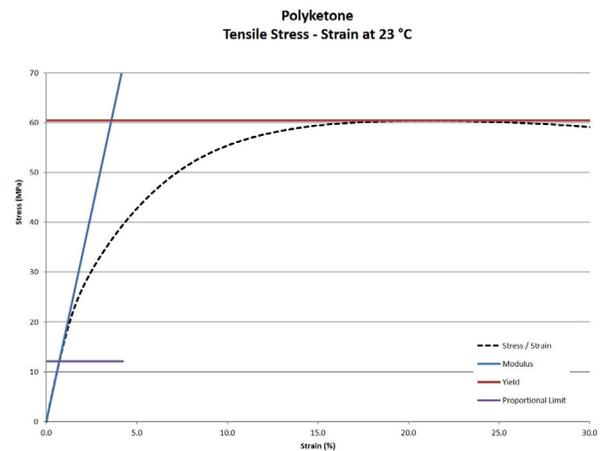
Figure 5. The tensile stress-strain curve is shown for the polyketone.
