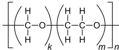
Figure 1. The structure of the polyacetal copolymer is shown.
