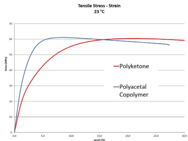
Figure 6. Overlay showing the stress-strain curves for the two materials.
