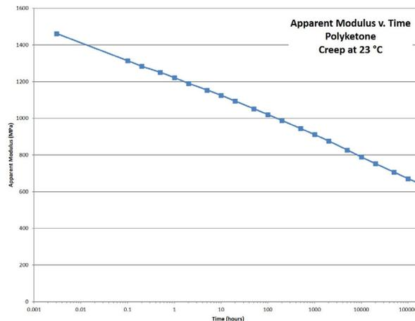
Figure 8. The plot of apparent modulus over time is shown for the polyketone.
