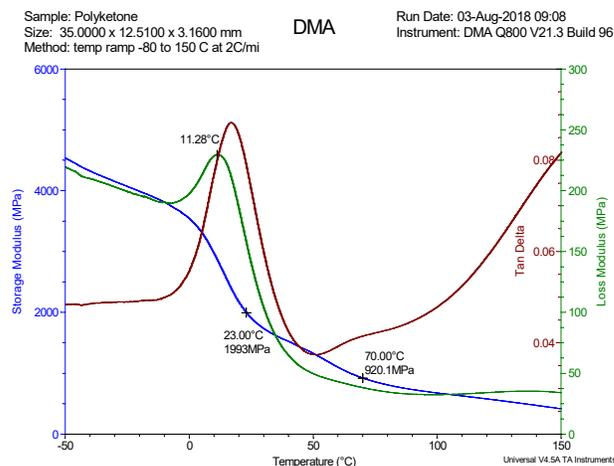
Figure 2. The DMA temperature sweep for the polyketone is presented.
