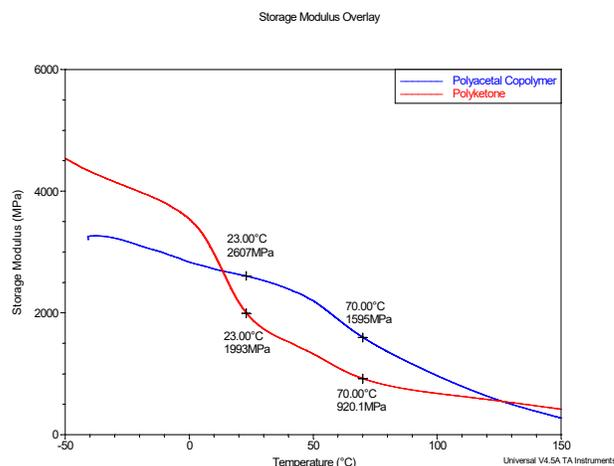
Figure 3. Overlay comparing the storage moduli of the two materials.
