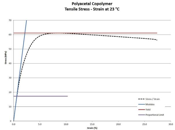
Figure 4. The tensile stress-strain curve is shown for the polyacetal copolymer.
