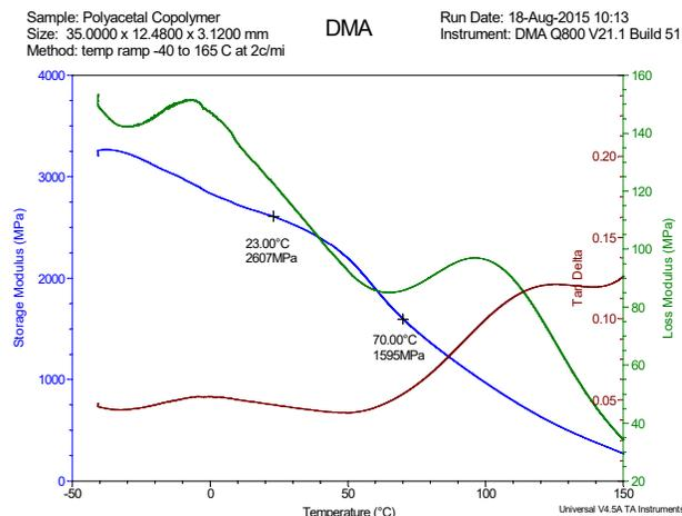
Figure 1. The DMA temperature sweep for the polyacetal copolymer is presented.
