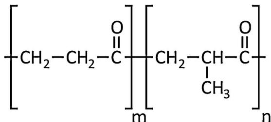
Figure 2. The structure of the polyketone terpolymer is shown.
