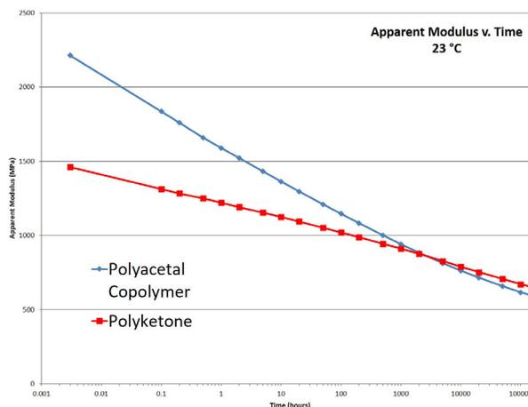
Figure 9. Overlay of the creep master curves for the two materials.
