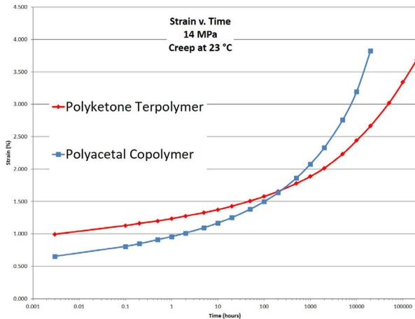
Figure 10. Plot of strain over time for the polyacetal copolymer and polyketone terpolymer.
