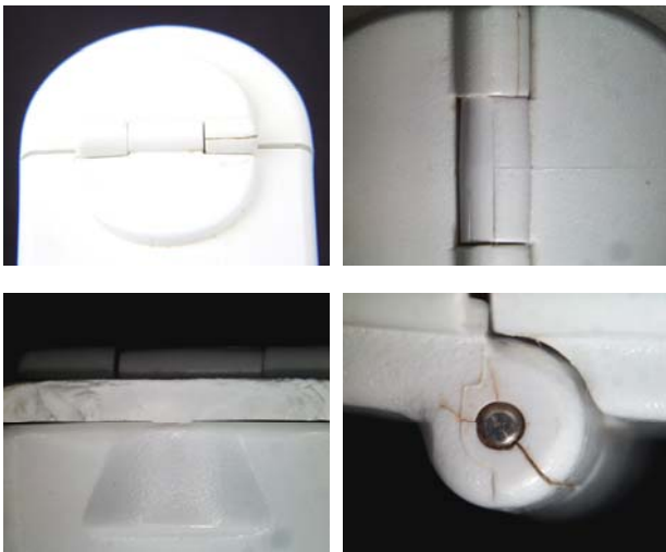
Fig. 1 - Cracking was present within the housing assembly
